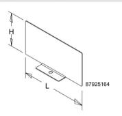
Used to divide a straight section splice into two sections. BULLETIN: F23
